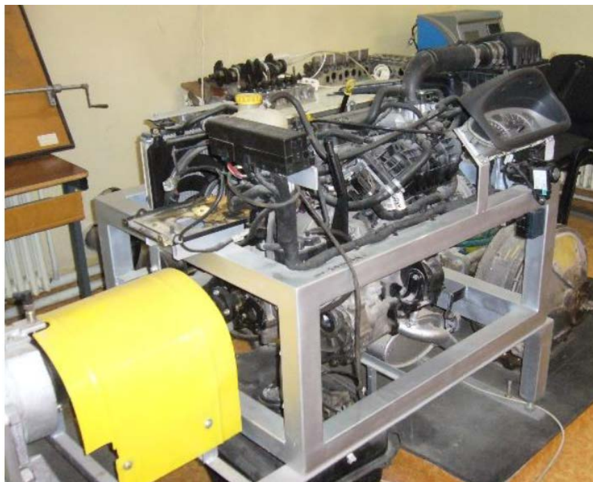
Figure 11. The test bed used to obtain the indicated diagram.
